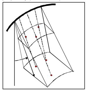
figure 6: determination of exterior orientation (including orbit in the scene area) just based on inclination, ellipse parameters and view direction
