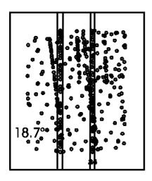
figure 5: Measured image points (image of December 24, 1996), line of tie points in the overlapping area of the sub-scenes
