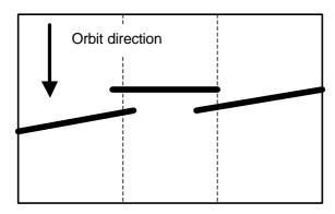
Figure 2: location of CCD-line-sensors in the image plane
