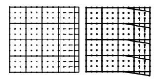
figure 8: effect of additional parameter 11 and 13 to image coordinates
