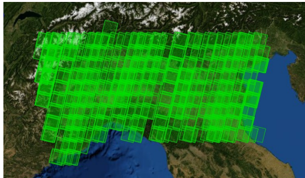
Figure 1: North Italy test area. The is covered by 414 Cartosat-1 stereo pairs, indicated by the green squares.
