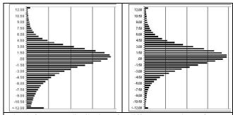
Fig. 4: frequency distribution of Z-differences against reference DEM – left: original matched DSM, right: filtered DSM negative: matched DSM is located above reference DEM
