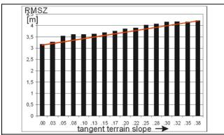
Fig. 5: root mean square discrepancies of generated DSM against reference DEM, as function of the terrain inclination; Mausanne, January after filtering  $SZ = 3.15m + 1.9 * tan \alpha$
