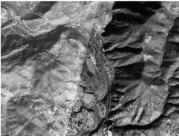
(c) Detail of orthoimage mosaic, showing the consistency of the independently processed scenes 115/208 and 116/208.
